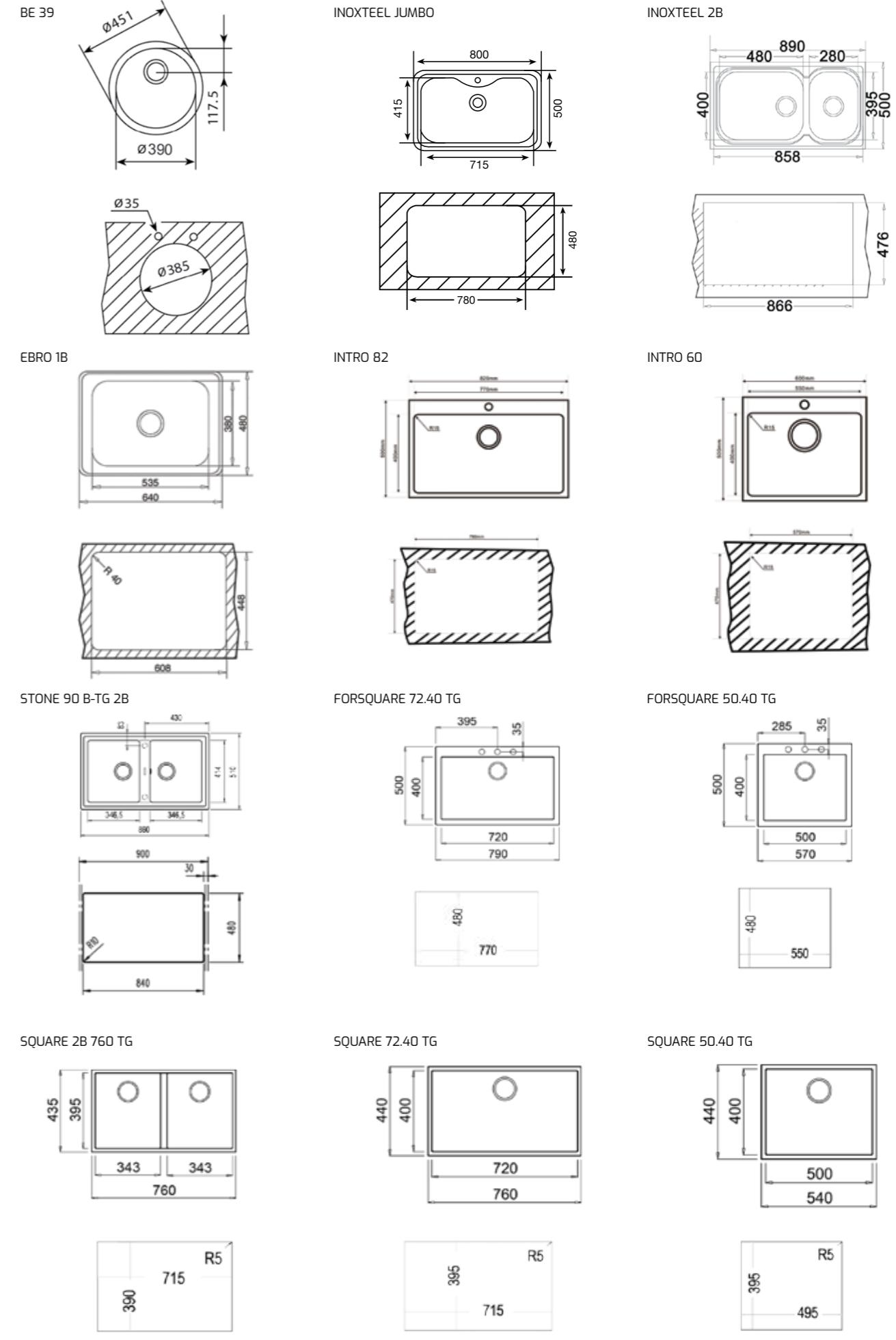
[D- Dimension (mm)] [BID - Built-in Dimension (mm)- (Length x Width x Depth)] [ED- External Dimension (mm)] [B- Bowl Dimension (mm)]
